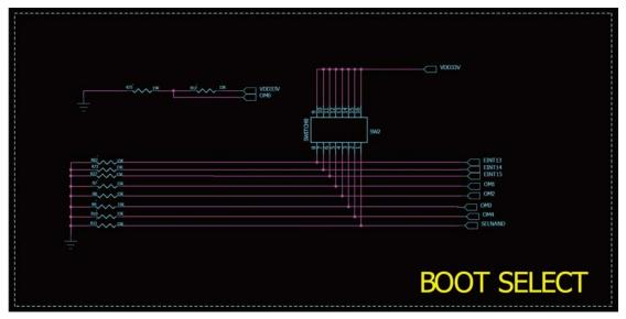
The OM0 is a signal that selects the clock source. When the OM0 is set as "0", XTlpll is selected as the clock source; while when the OM0 is set as "1", EXTCLK is selected. On the TE6410 SBC we selected XTlpll.
