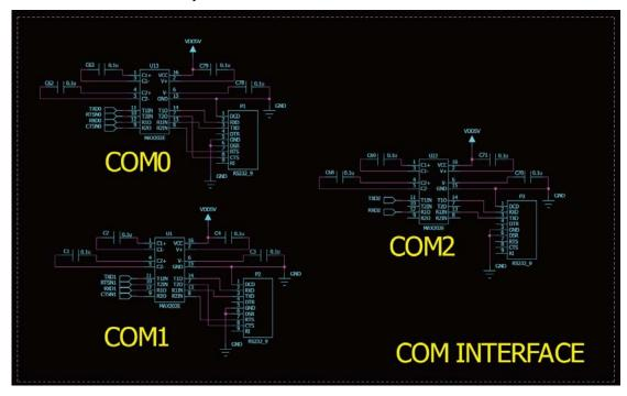
Schematics of the serial ports are shown as below:
